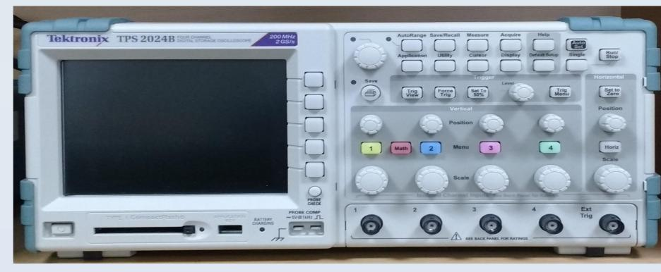
Four Channel Isolated Digital Storage Oscilloscope
